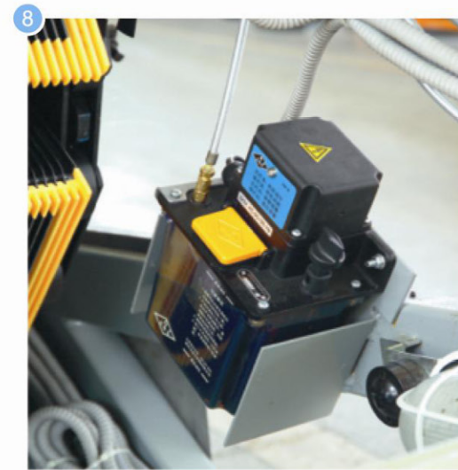
8. Oil refill automatically by AI computer control for chain lubrication.
