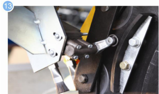
13. Mechanical type unintentional reversal travel direction.
