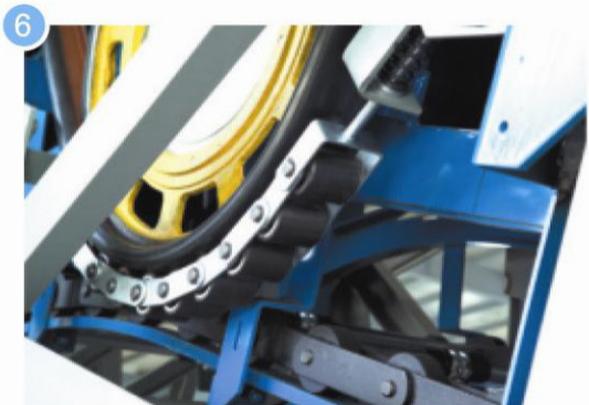
6. Aluminum- core rubber wheels for handrail belt can equally divide the force under stress, and maintain a long-life motion.
